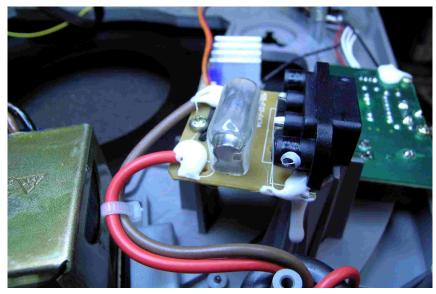
Step 2) Locate power receptacle. The fuse is covered with a soft plastic insulator.
