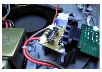
Step 3) Remove the insulator to reveal the fuse.
