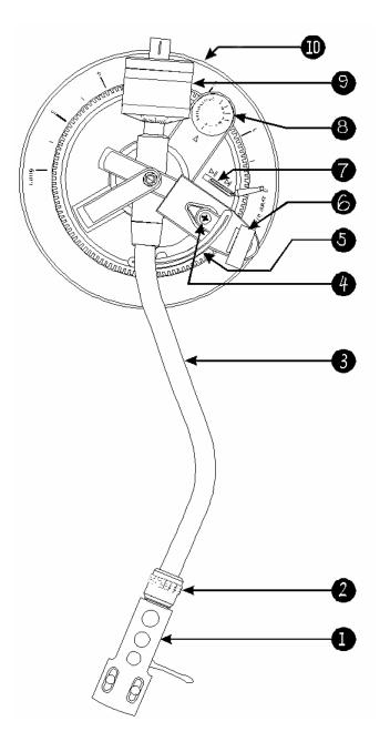
**1. Headshell -** Install cartridge here. When installing a cartridge, refer to the installation instructions supplied by the manufacturer of that cartridge. During installation, attach the stylus protector to guard the stylus tip from damage. Attach wires as follows:
