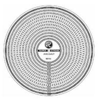
Half speed mastering of 78s is possible, by setting the pitch control to its 20% range and the main speed to 45. Then, adjust the pitch control using the "78" section of the supplied strobe disc to obtain 39.13 rpm.
