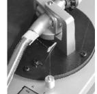
**10. Tonearm Height** – Adjustment is by *knurled ring* at arm base. It is calibrated 0 to 6 mm. Unlock knurled ring by turning lock lever (10) counter-clockwise (in picture it is hidden by item 9). Then adjust knurled ring counter-clockwise to raise arm, clockwise to lower arm. If you require 14 inch disc capacity, adjust arm height to obtain clearance at item 4. Usually this setting is at 1.5 mm (this varies with cartridge used). When done, turn lock lever to "lock."
