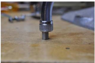
Use a metal spacer and push the rubber connector into by the distance of the headshell connector length + a fraction of an inch. Maybe 1/32." Be carefully so that it is only deep enough to permit the headshell to fit in easily. CAUTION: DON'T PUSH IT TOO FAR IN. If you do, you have to start all over again! Do this is small portions tweak and check until you have it in only the sufficient distance.
