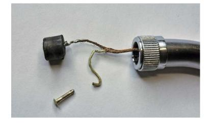
The ground wire connected to one pin goes. Not needed anymore.
