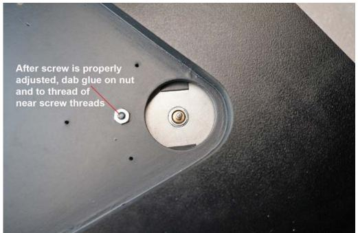
motor flange will be 1/8" above the deck. When satisfied that the motor is attached evenly on both ends, smear a bit of Duco cement or Elmers's Glue-All over the nut top and nearby screw threads.
