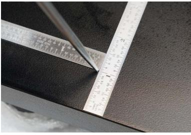
Use an awl to mark the spot to drill for the switch. It will be on the top front left.
