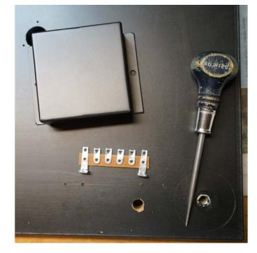
Drill an additional 5/64" pilot hole 3/8" deep at 7" from the front lip, and 3-7/8" from the bottom right. This is for the cable clamp. Refer to final bottom picture.
