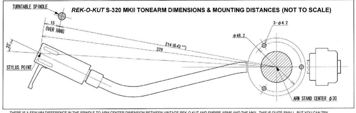
THERE IS A FEW MM DIFFERENCE IN THE SPINDLE TO ARM CENTER DIMENSION BETWEEN VINTAGE REK-O-KUT AND EMPIRE ARMS AND THE MKII. THIS IS QUITE SMALL, BUT YOU CAN TRY TEMPORARILY POSITIONING THE MKII AT THE OLD MOUNTING POSITION AND USE A CARTRIDGE ALIGNMENT GAUGE TO CHECK IF ALL IS OK. THERE IS PLENTY OF ADJUSTMENT RANGE BUILT INTO THE HEADSHELL SLOTS. TRY TO ACHIEVE THE 15 MM OVERHANG AT STYLUS TIP. WITH EMPIRE 598, MOUNT CARTRIDGE TOWARDS BACK. OTHERWISE, MOUNT THE MKII AT THE 8.43 DISTANCED.
