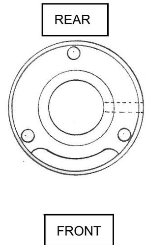
2. Mount the arm base to the turntable base with the routed-out quarter moon facing the front of the base. To do this you must drill a 1.25" hole in the base and provide three holes for the mounting screws.
