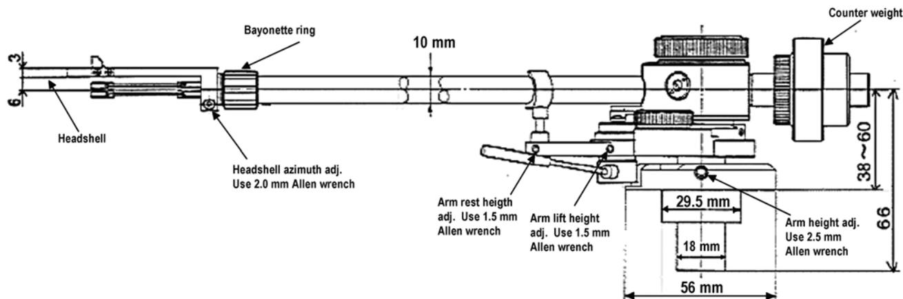
9. If necessary, adjust the height of the arm rest with the appropriate hex set screw. If playing 16" transcriptions, (Transcribe and S-240 only) you may want to carefully shorten the plastic projection at the arm rest's bottom.
