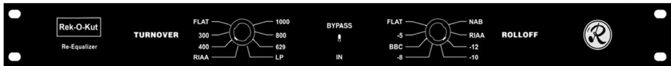
The front panel has three controls: Turnover, Rolloff, and Bypass. The Turnover has eight positions: FLAT, 300 Hz, 400 Hz, RIAA, Lp, 629 Hz, 800 Hz, and 1000 Hz. The Rolloff also has eight positions: FLAT, -5 db, BBC, -8 dB, -10 db, -12 db, RIAA, and NAB. The BYPASS switch provides a hard wire connection from input to output with no intervening circuitry. When switched to "IN," the two inputs are connected together providing mono operation. This reduces some noise and facilitates recording.
