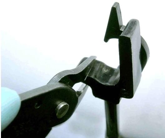
What has to be done is to carefully line up the cutting edges of the tool with the protrusion which interferes with setting the arm at the edge of the record. You must cut just after the "U" shape of the arm lift. See the illustration at the left.
