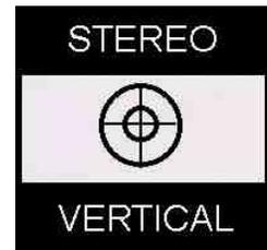
Another use for this switch is to remove the solo performer or soloist from stereo recordings. This works only if that performer is in the center field of the recording. Also, to perform this, the “mode” switch of the amplifier must be set to “mono,” or the output of the turntable must be combined with a “Y” connector.
