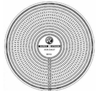
Half speed mastering of 78s is possible, by setting the pitch control to its 20% range and the main speed to 45. Then, adjust the pitch control using the “78” section of the supplied strobe disc to obtain 39.13 rpm.
