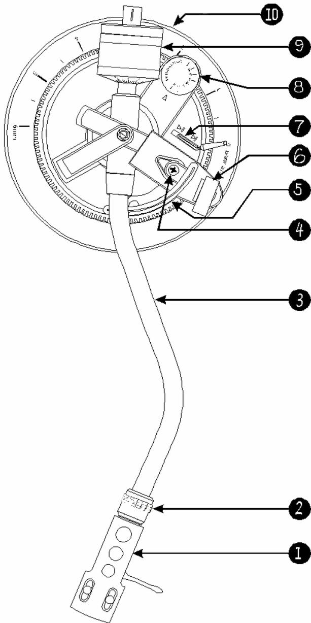
**1. Headshell** - Install cartridge here. When installing a cartridge, refer to the installation instructions supplied by the manufacturer of that cartridge. During installation, attach the stylus protector to guard the stylus tip from damage. Attach wires as follows:
