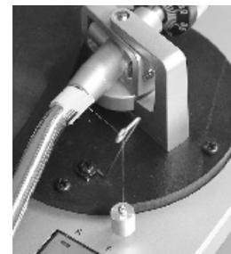
**10. Tonearm Height** – Adjustment is by *knurled ring* at arm base. It is calibrated 0 to 6 mm. Unlock knurled ring by turning lock lever (10) counter-clockwise (in picture it is hidden by item 9). Then adjust knurled ring counter-clockwise to raise arm, clockwise to lower arm. If you require 14 inch disc capacity, adjust arm height to obtain clearance at item 4. Usually this setting is at 1.5 mm (this varies with cartridge used). When done, turn lock lever to "lock."
